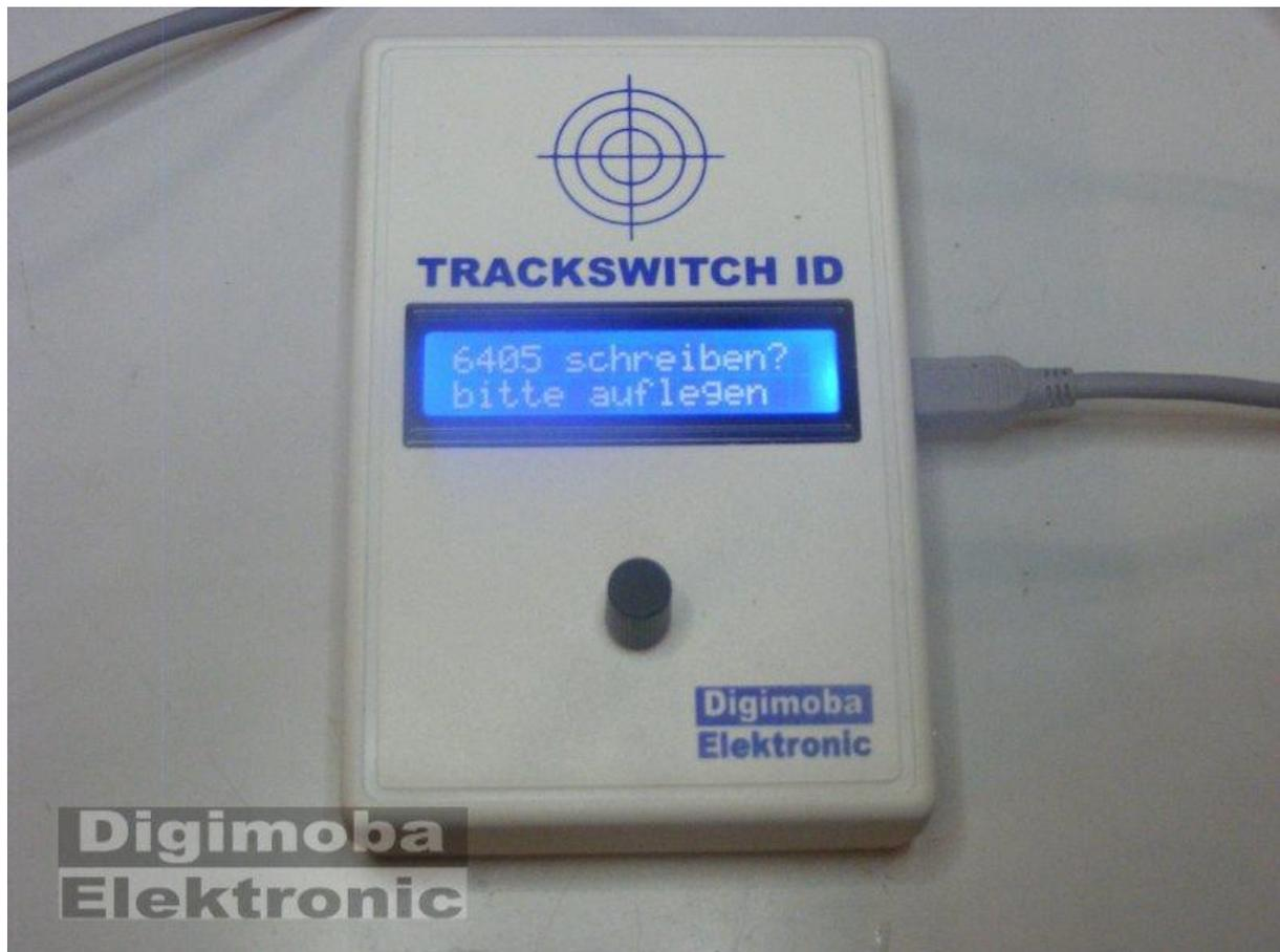
The Trackswitch ID Manager is used to read and write RFID Tags, also called transponders. These transponders are available in various forms. Transponders in paper or in foil form are ideally suited as stickers for model railway purpose.
